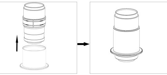
3. Insert the gear ring of the C100IS-F on the plastic c-ring, as shown in the diagram, until it reaches the flange of the plastic c-ring.
