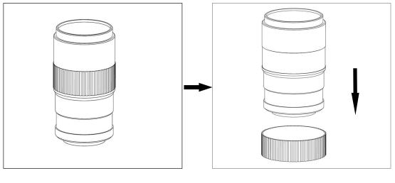
Remove the rubber ring from the lens carefully.
