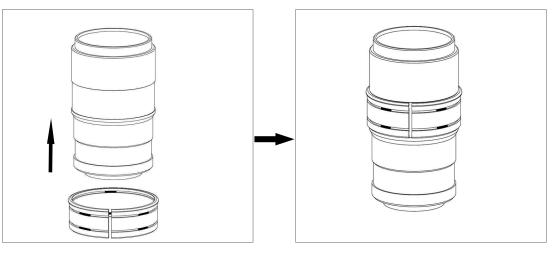
2. Insert the plastic c-ring of the C100IS-F onto the rubber ring recess of the lens.
